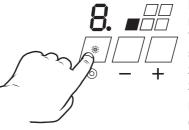
Press the cooking zone symbol next to the plus/minus sensor. The light on the left below the symbol for the dual-circuit-cooking zone indicates that the cooking zone has been activated.
